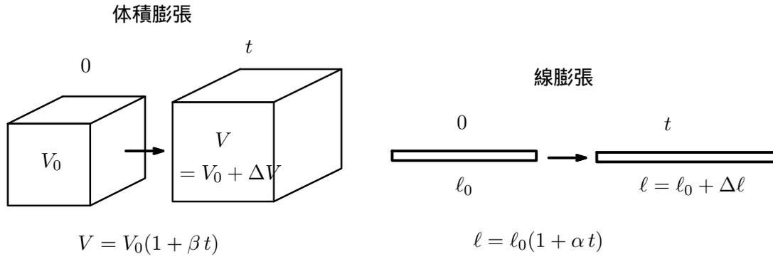
$$\Delta V = V - V_0 = (l_0 + \Delta l)^3 - l_0^3 \simeq 3 l_0^2 \Delta l$$
