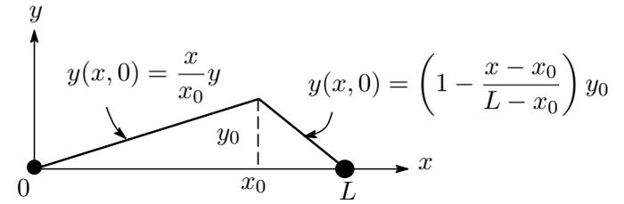
$$\left(\frac{\partial y(x, t)}{\partial t}\right)_{t=0} = 0 \quad (t = 0 \text{ で弦は静止}) \quad (8)$$
